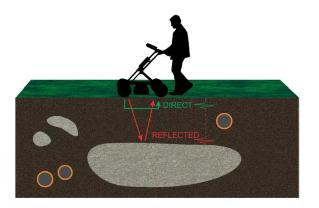
Data is collected in parallel lines in a **grid layout** using tapes and ropes to guide the operator and to ensure the entire area is covered. Ground-based GPR units are dragged or pushed along the ground,
