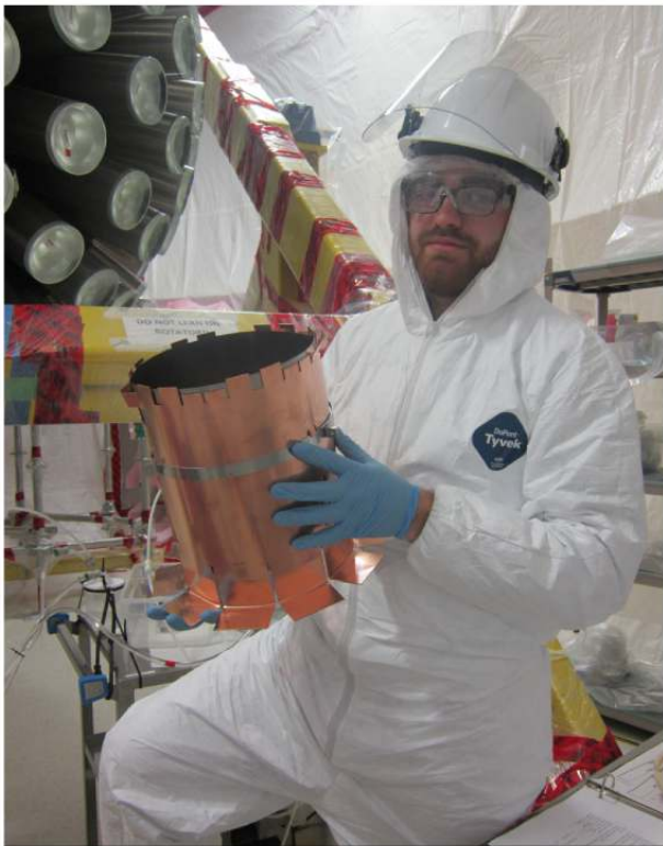
Copper thermal shorts keep the PMTs at the right temp.
