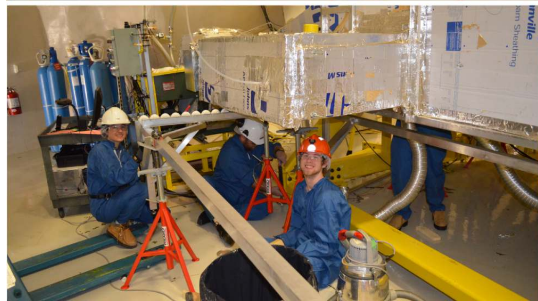
The AV is heated up for the fifth time to harden and relieve stress in the LG bonds.
