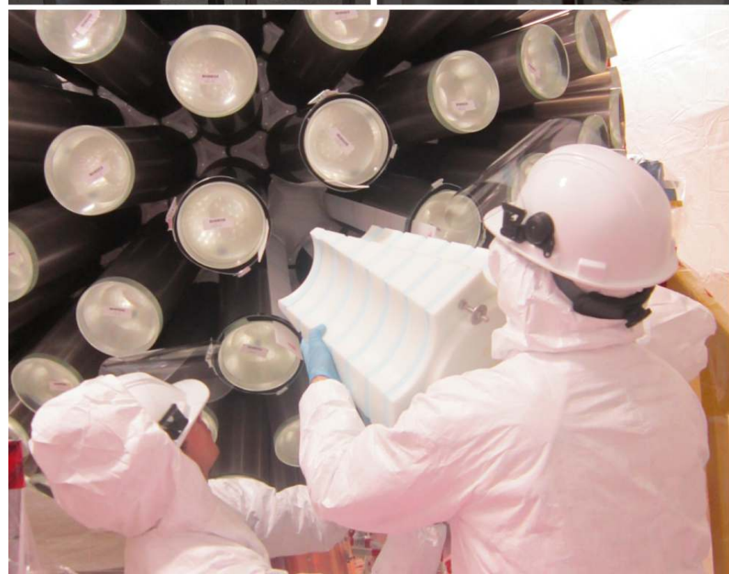
Fillerblocks, made from layers of blue foam
