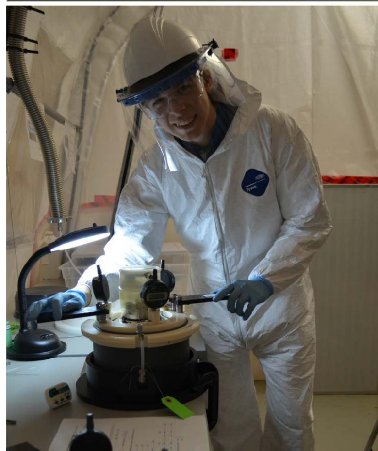
Fully mounted PMT. Two green tags indicate it passed the pressure and the Helium leak test.
