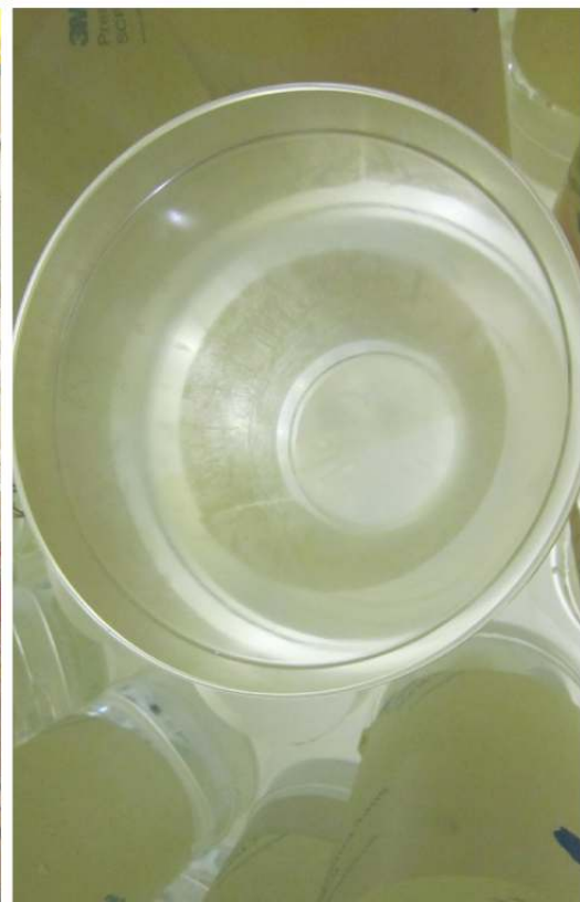
After the bonding syrup is polymerized, the bond is locally heated to harden it.
