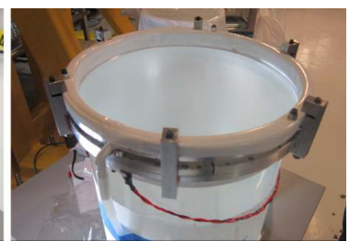
Dam and clamps in place, ready for bonding.
