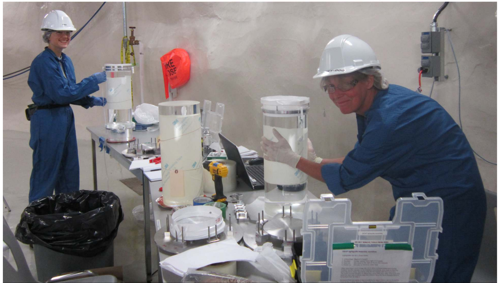
Dams and clamps are installed on the light guides (LGs). The clamps seal the dam against the acrylic of the LG and later the stub, confining the bonding syrup to the gap between them until it hardens.
