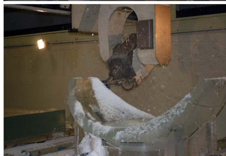
The sheets are thermoformed and machined into 'orange slices'.
