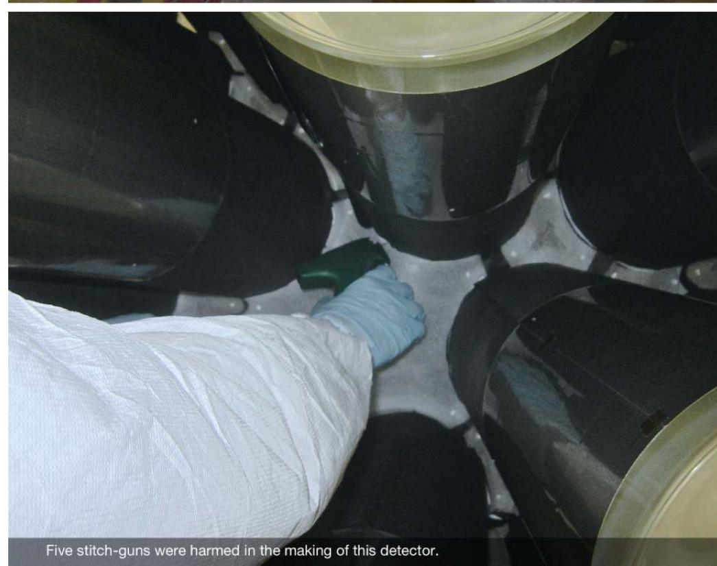
Specular reflector and magnetic shielding are wrapped around the LGs.
