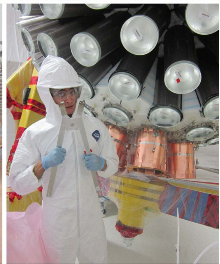
Not a tool used in dentistry, but a spring stretcher.
