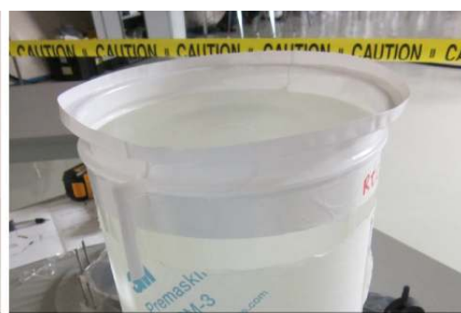
The dam will keep the glue from flowing away.
