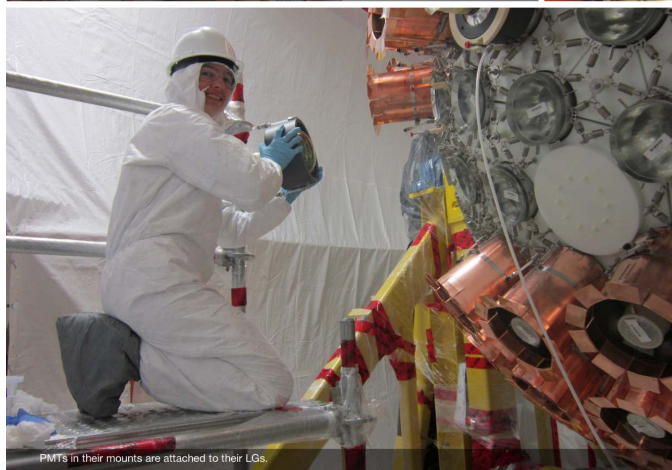
A PMT secured to the AV for the pressure test to verify adequate o-ring seal to the LG.
