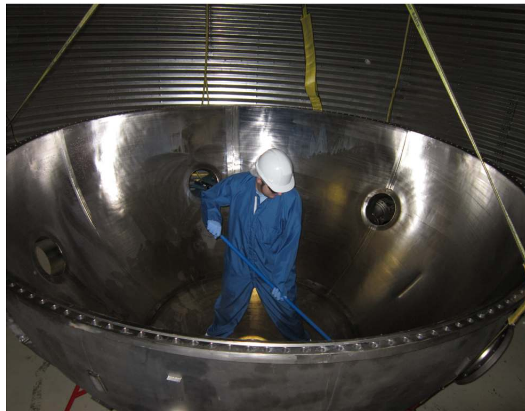
Washing the stainless steel shell.
