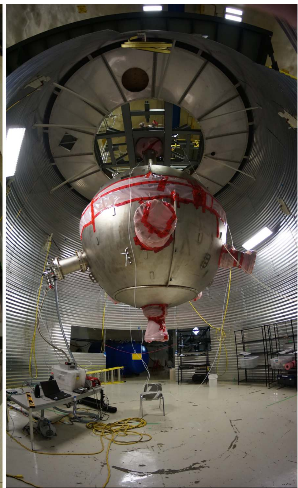
The stainless steel shell ready for leak testing.
