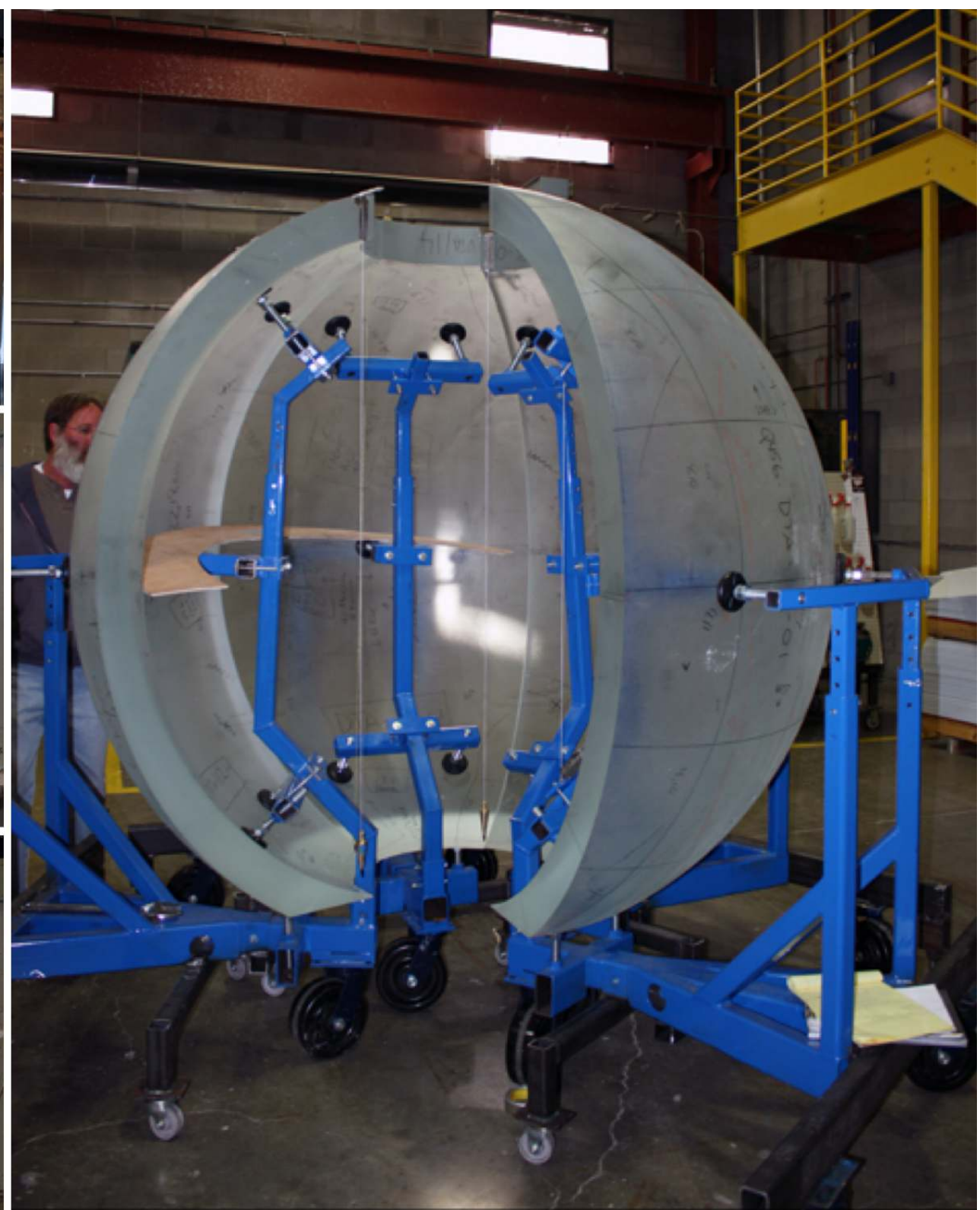
The 'orange slices' are dry-fit before being bonded together at Reynolds Polymer Technology, Inc.
