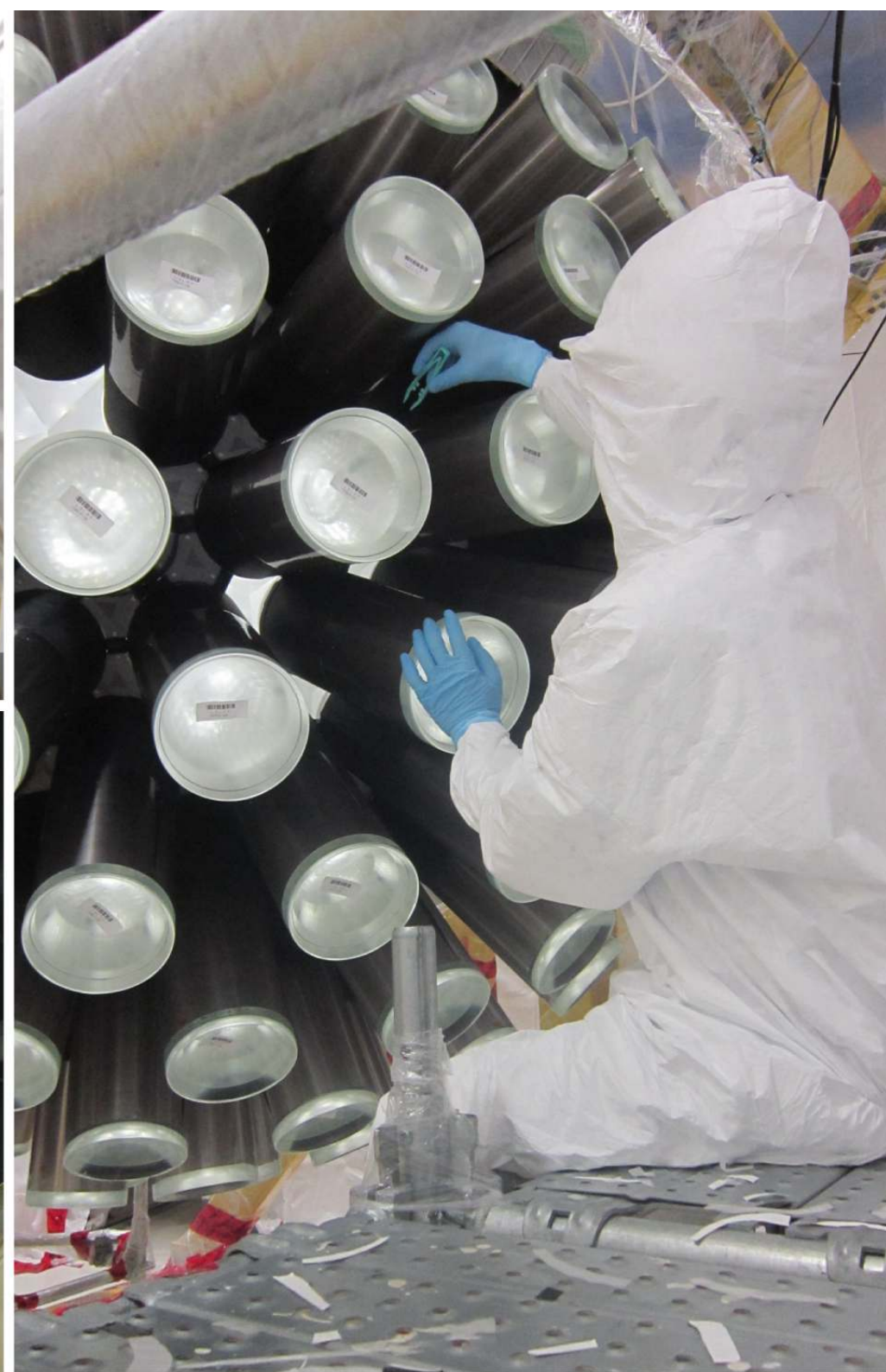
Diffuse reflector pieces are stitched together to cover the facets between the LGs.
