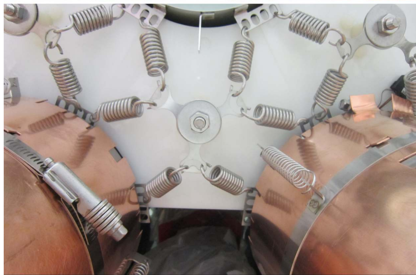
Spring keeps filler blocks in place while allowing them to move during cool-down.
