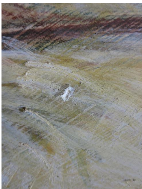
Figures 8 and 9 show damage to the paint layer from disruption in the underlying Plaster due to possible changes of hydration states of salts contained in the plaster.
