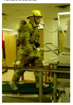
Peak oxygen uptake (VO<sub>2peak</sub>) will be measured during a progressive, incremental exercise test to exhaustion on a treadmill.
