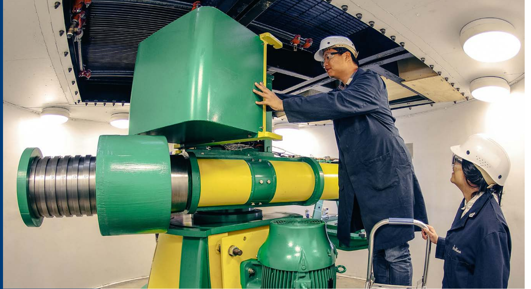
The Geomechanical Centrifuge Experimental Research Facility boasts a 50g ton beam centrifuge.
