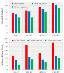
insulation layers. A stiffness reduction of due to the insulation was observed (bottom figure). Concrete crushing combined with wood embedment was the dominant failure observed for specimens with insulation. The specimens without insulation showed screw yielding along with wood embedment.
