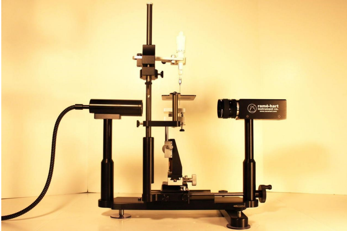
Figure 3.7 Ramé-Hart Goniometer Model 250 Setup. 8
