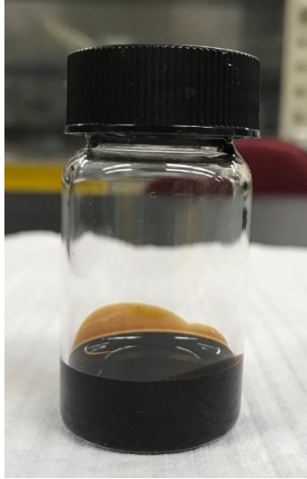
Figure 3.2: A glass vial containing opaque mixture of asphaltene + polystyrene + toluene.
