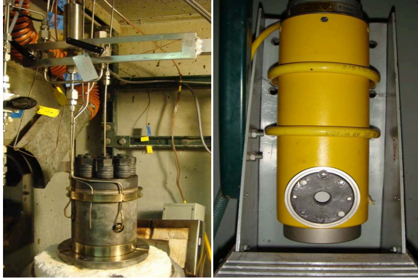
Figure 14: (Photo on the Left) Assembled View Cell, (Photo on the Right) X-ray source
