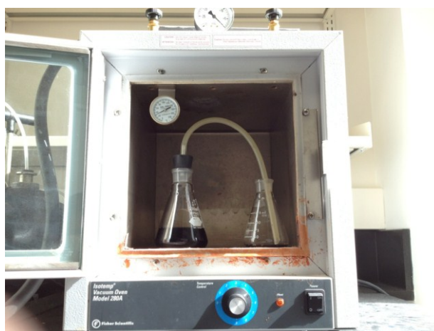
Figure 2-2 Photo of “Froth Treatment” Reactor and heating system
