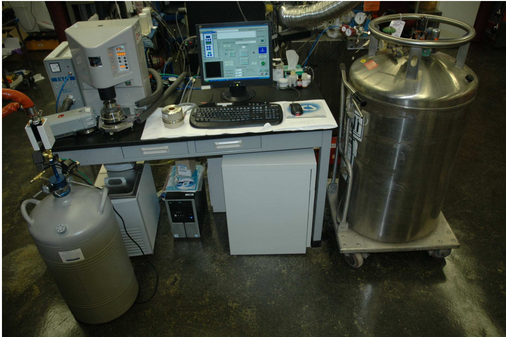
Fig. A.6. Experimental set up for measurement of rheological properties.
