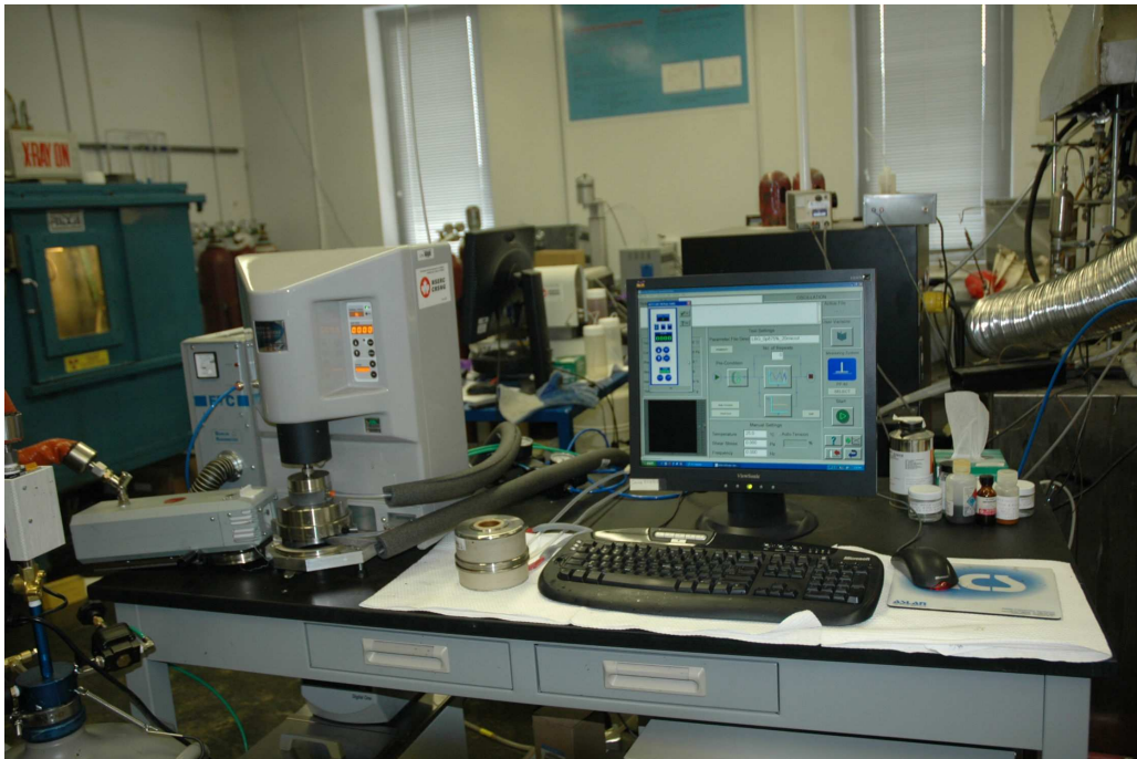
Fig. A.7. Experimental set up with peltier plate assembly for rheological measurements.
