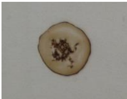
Figure 3-7 Dried flocs from the aged Nexen FWKO subsample A.
