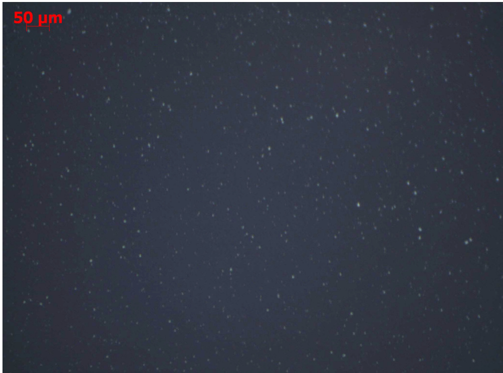
Figure 3-19. Mesophase formation in the stirred hot-stage reactor with the block magnet. Mesophase particles are uniformly distributed over the window after turning off the stirrer.
