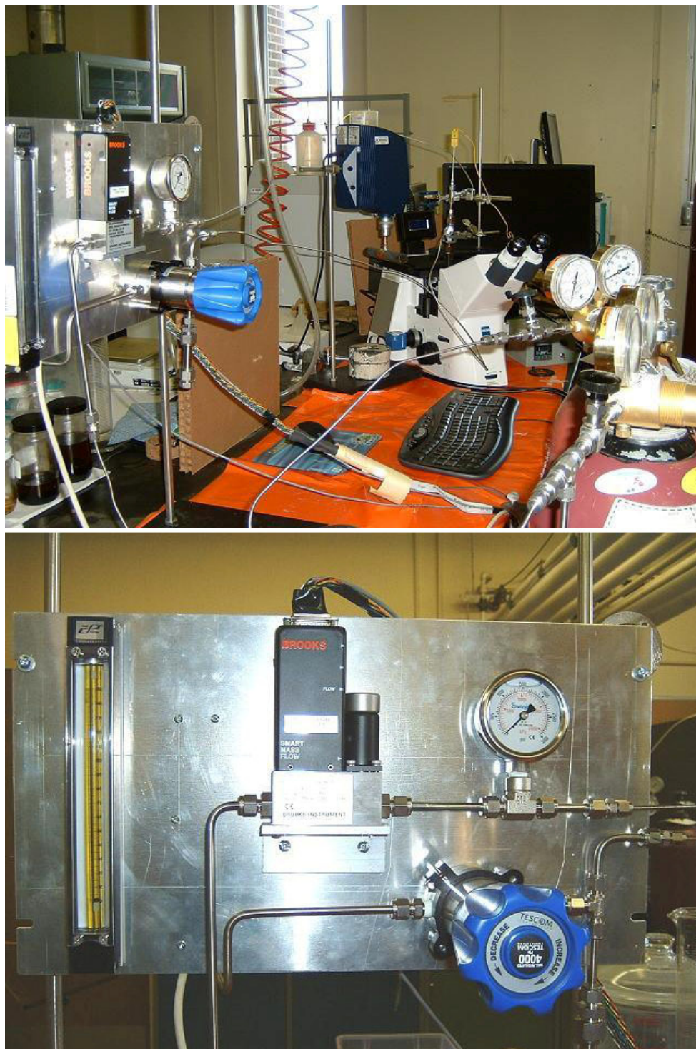
Figure 3-22. Set-up for the continuous flow of gas inside the hot-stage.
