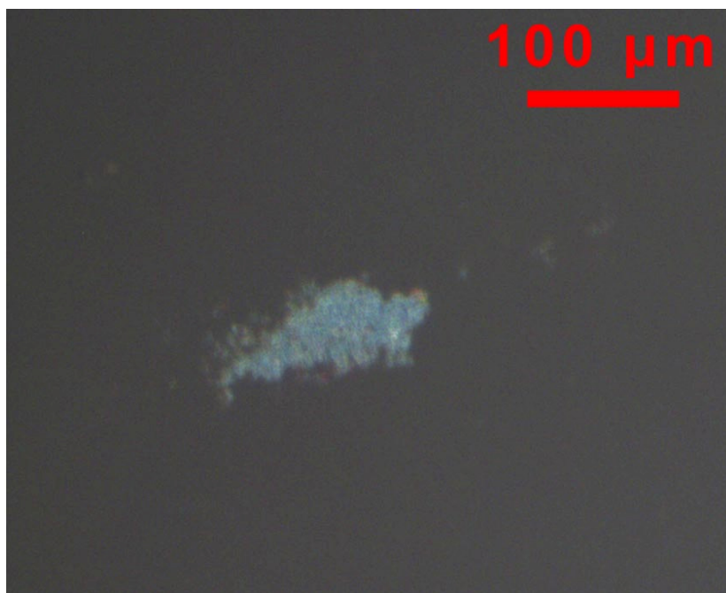
Figure 5-4. Photomicrograph of initial mesophase observed during cracking Athabasca bitumen under hydrogen at 4.8 MPa and 440°C with agitation at 140 rpm as an aggregated domain.
