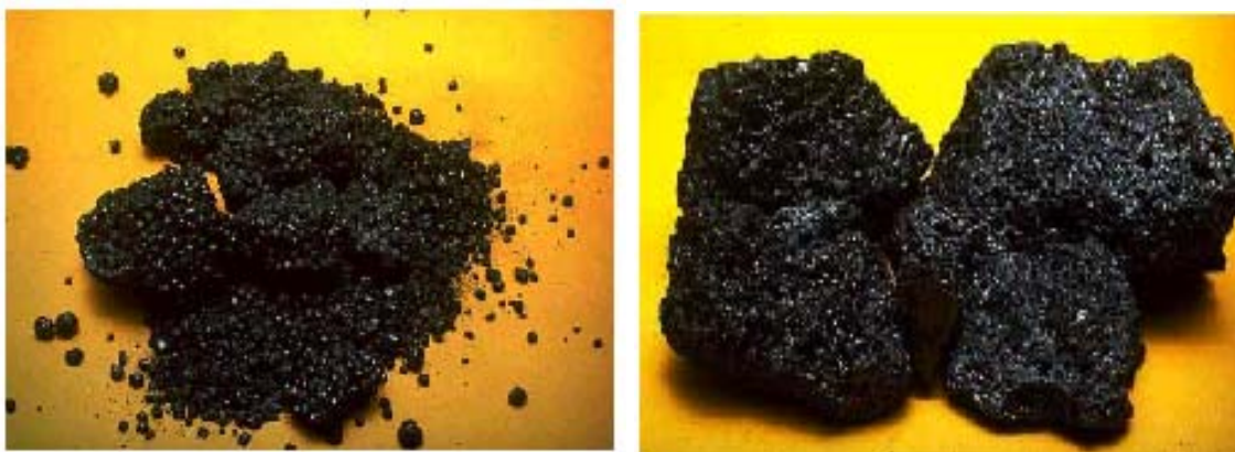
Figure 1.2: Samples of different cokes obtained from vacuum residue processing. Left: shot coke. Right: sponge coke (Elliot, 2001).
