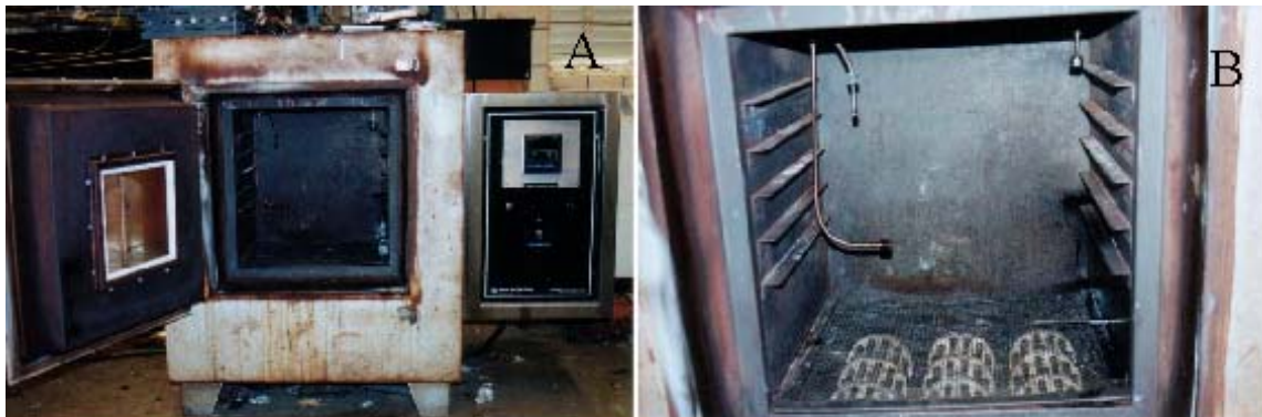
Figure B-1: Pictures showing the electric furnace. A: general view. B: detail of the heating camera with the tubing to connect the coker.
