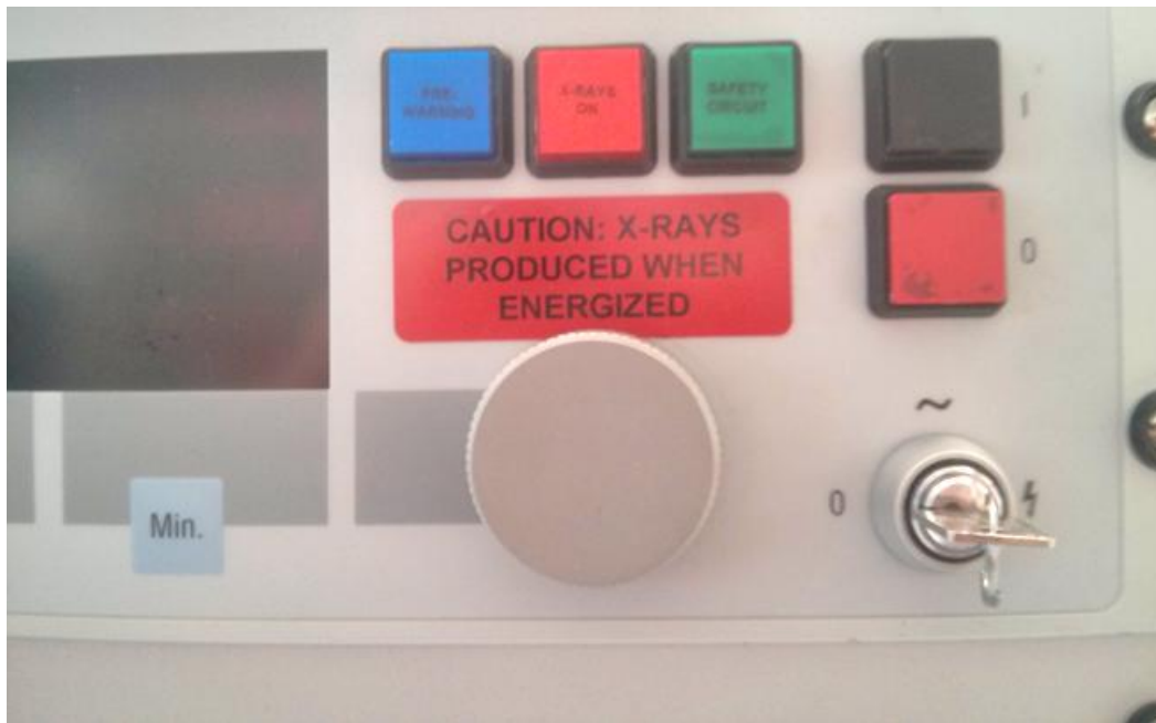
Figure 1. The x-ray control panel (XYLON panel). (0), (~) and (⚡) represent OFF, STANDBY and ON positions respectively.
