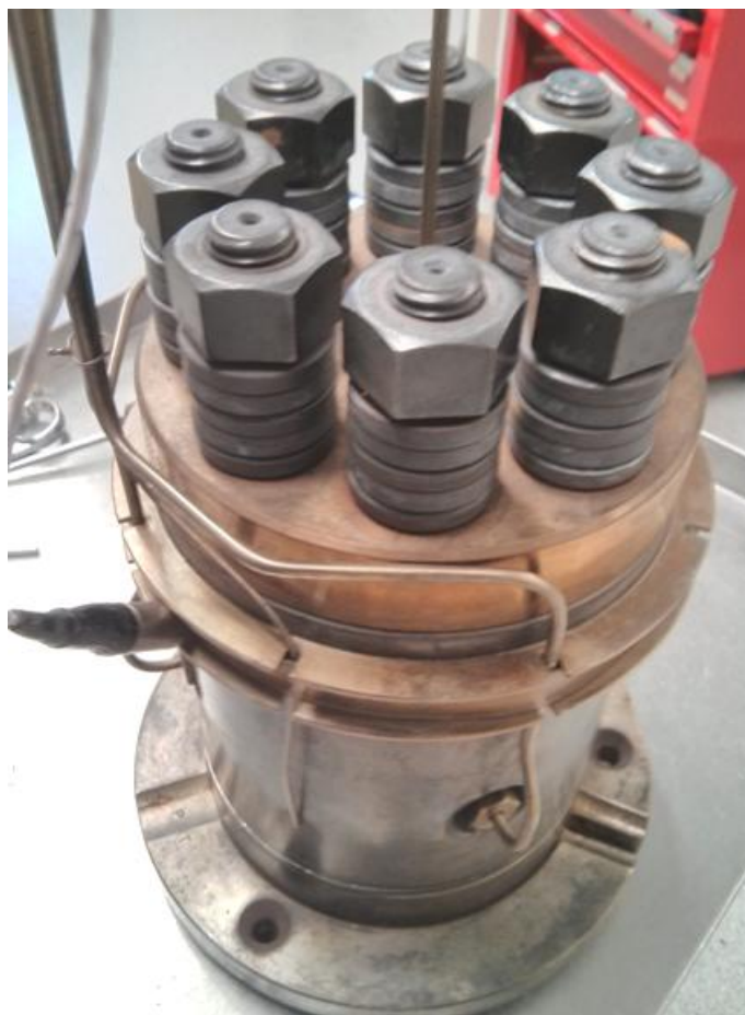
Figure 3. Correct position of the beryllium cell with respect to the cell mount
