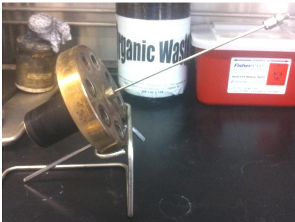
Figure 11. Designated structure to protect the bellows cap.
