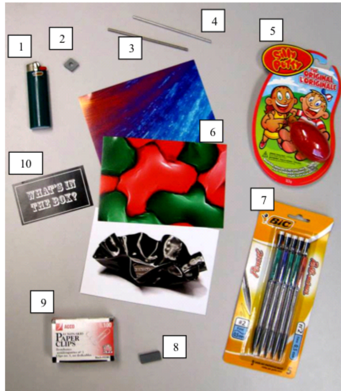
Figure 4. The “What’s in the Box?” box and its contents: 1) Lighter, 2) Ceramic cutting tool insert. 3) Alloy 6061-T6 rod, 4) Alloy 1100 rod, 5) Egg of Silly Putty™, 6) Set of 3 postcards of various materials with descriptions on the back, 7) Mechanical pencils, 8) Bar magnet, 9) Box of 100 paper clips, 10) “What’s in the Box?” sticker. Photos © John A. Nychka 2010, 2011.
