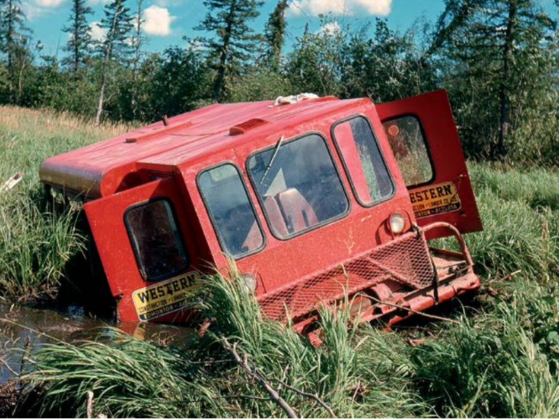
Photos taken by Gordon Berdahl chronicle the process of building a highway, circa 1963. Above left, a tracked all terrain vehicle, often referred to as a “swamp buggy” is mired in a beaver dam on the route of Highway 63. This type of vehicle was often used to access locations ahead of actual construction in the unfrozen summer period. Right: this photo, also in the summer of 1963, shows the first piece of Highway 63 subgrade construction underway about 5 kilometres north of Wandering River.
