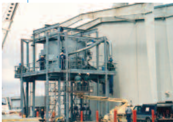
Ritter designed a full-scale unit built at the hazardous waste disposal site in Swan Hills, Alberta. The unit (above) was used in the decontamination of PCB-laden transformers. Below, Ritter is seen with a pilot model of a process that was used to destroy tons of war chemicals at Canadian Forces Base Suffield, in southern Alberta.
