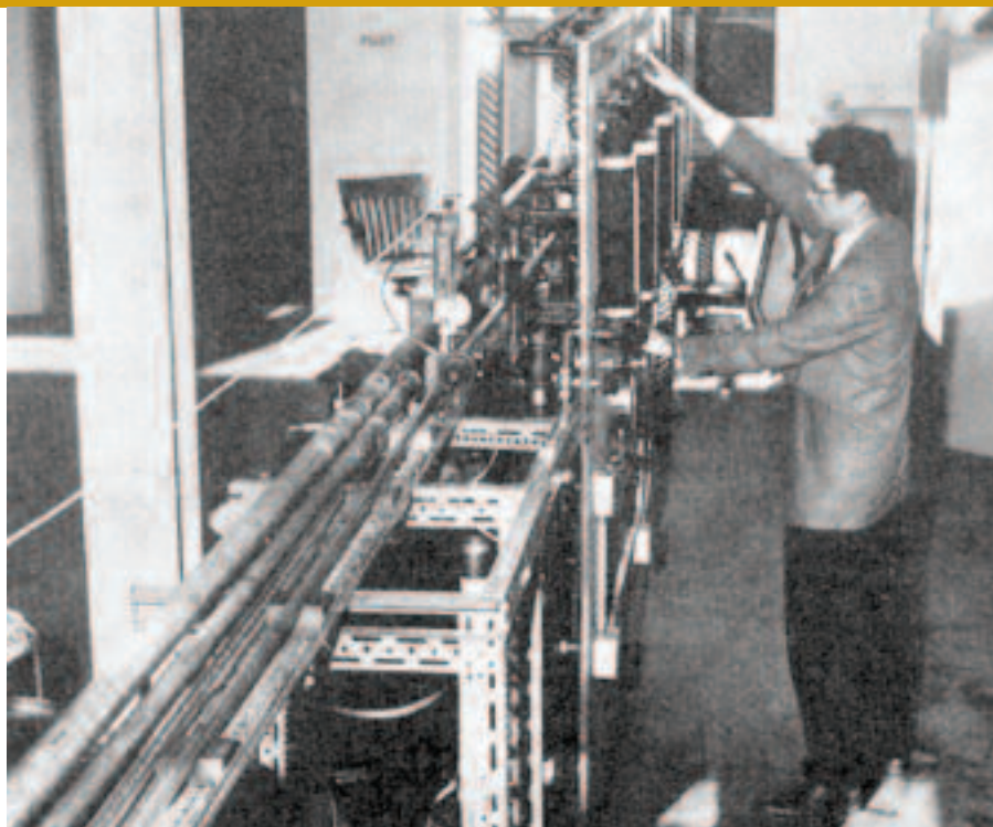
Working at Alberta Research Council in 1957, Russell adjusts the pilot pipeline used to study oil to water flow. EDITOR'S NOTE: This photo is taken from the book Athabasca Oil Sands – From Laboratory to Production by Mary Clark Sheppard, published by Geoscience Publishing.
