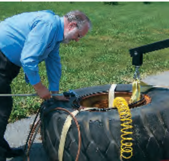
In Dr. Hahn’s first appearance as an expert witness, he tested and measured the lock and steel components of an off-road construction vehicle to determine reasons for tire failure.
