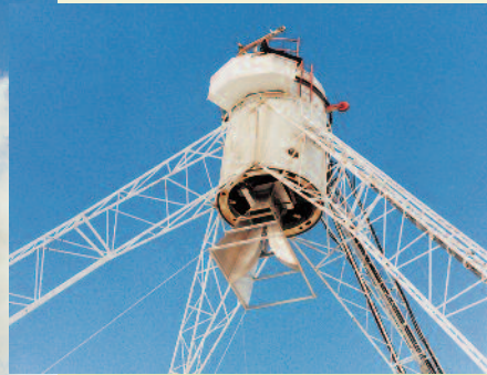
Below: The ridged feed horn just after it had first been installed at the feed point.
