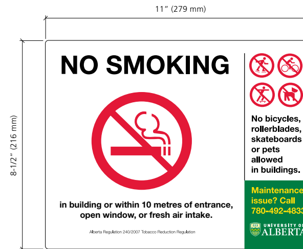
ST 3.9 North/South Campus Exterior No Smoking Sign/Decal w/ QA contact number. Item is two-sided with the adhesive design on back flipped to minimize show-through.
