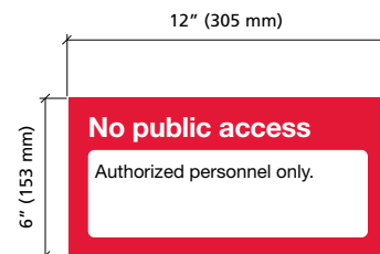
ST 2.9 Door Access Information Sign
