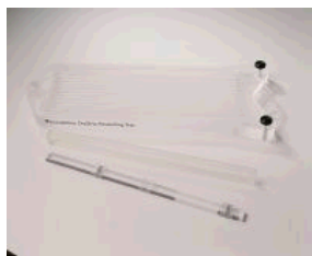
Fig 4-1. IPGphor Cup Loading Strip Holder (bottom) and 24 cm Immobiline DryStrip Reswelling Tray (top) for use with Immobiline DryStrip gels.
