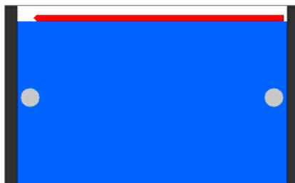
Fig 6-2. Diagram showing the preferred position of reference markers on the gel backing, with the gel backing lowermost.
