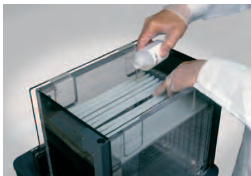
Fig 35. Spreading the tubing elements apart with one hand while pouring the solution with the other (to avoid pouring the 100× anode buffer onto the tubing).
