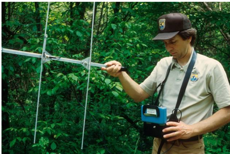
Figure 1: Person holding radio telemetric equipment (receiver with attached Yagi antenna). Image courtesy of http://elte.prompt.hu/sites/default/files/tananyagok/EthologyPractical/ch19s02.html
